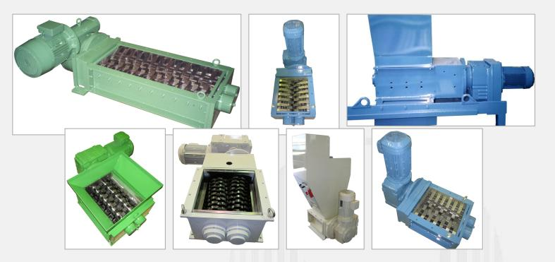
Crusher is feature by a series of knives assembled on two parallel shafts with opposite rotating direction.
