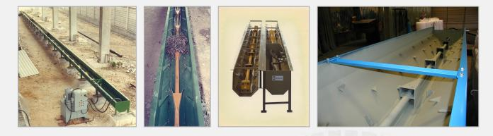
A spiked bar moving back and forth in a half-pipe with opposite directed spikes enables to move forward all kind of metal chips. Ideal for large quantities and flows. Can be placed in or out of ground.
