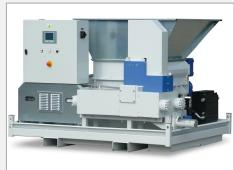
Recovering coolantVolume reduction Chips valorizationImplantation in a processing line of chips Flow rate: 50 to 1000 kg/h chips
